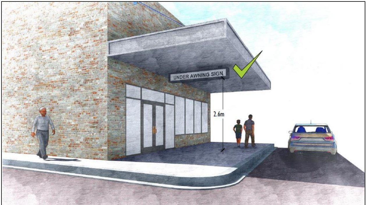
Figure 13: Under Awning Signage
