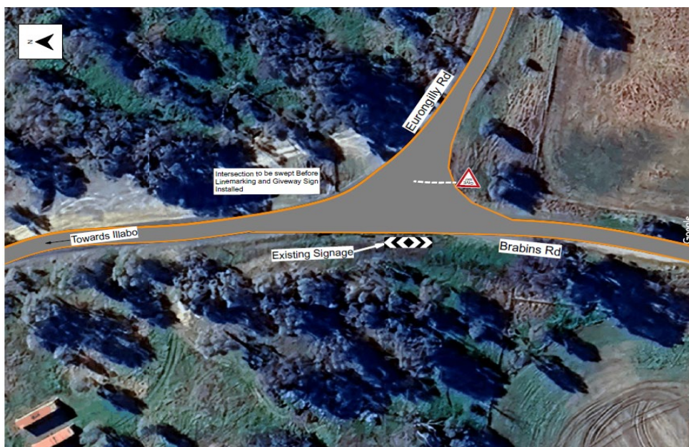
Figure 5: Give way Sign Eurongilly-Brabins Road intersection
